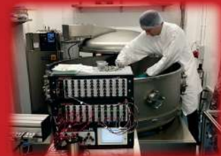
TVAC in a Cleanroom
